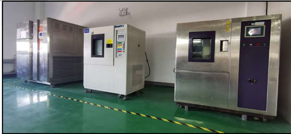
高低温冲击实验柜,恒温恒湿老化实验 High and low temperature impact test cabinet, constant temperature and humidity aging test cabinet
